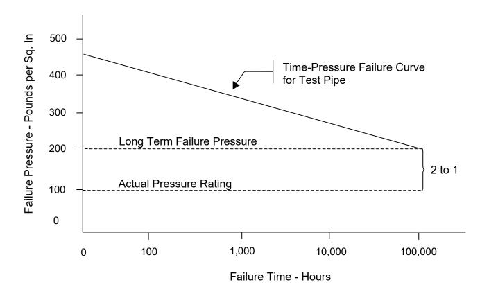
The figure above illustrates the basic method used in assigning Pressure Rating.
